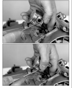
Lean the engine to the left and take out the wrist pin's RH snap ring.
